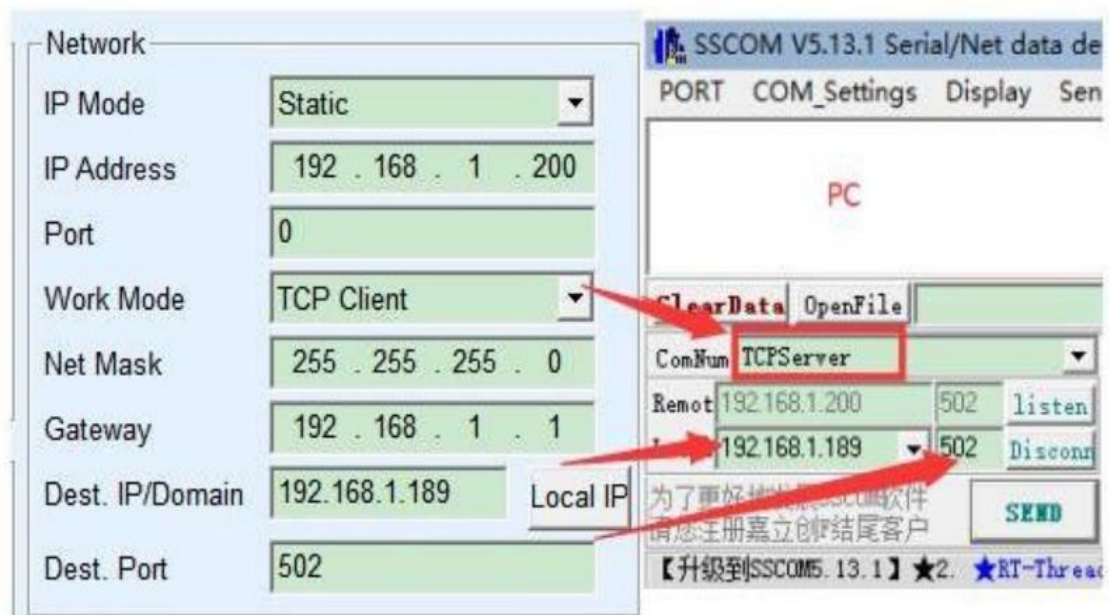
Figure 20 Serial server as a client
