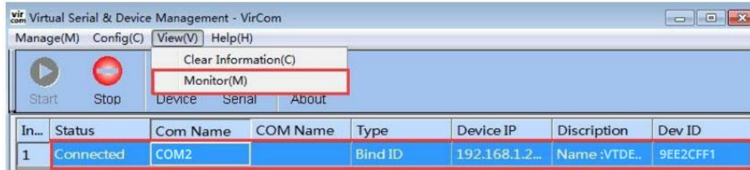
Figure 32 Open Vircom monitoring
